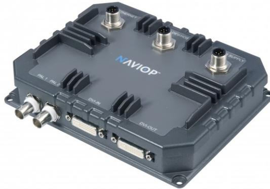
**The SHARP VIDEO unit** is the core of the “integrated glass bridge” and NAVIOP GEN3 visualization system based on WindowsCE 6.0 R2 Operative system and NAVIOP NMADE (runtime) application software.
